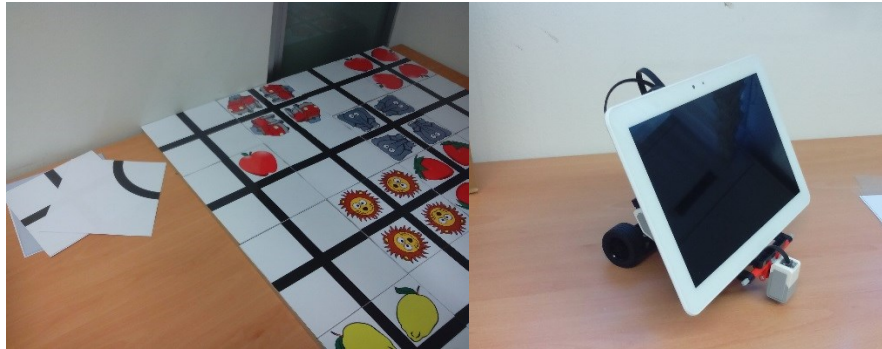
Fig. 2. The tangible surface's parts. On the left, the different tiles that compose the physical surface. On the right, the mobile robot that displays the digital content
