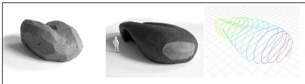
Figure 8: Form finding and the digital model of an example design, Herkrath, Lohmann, Pofahl, Chair of structures, RWTH University.
