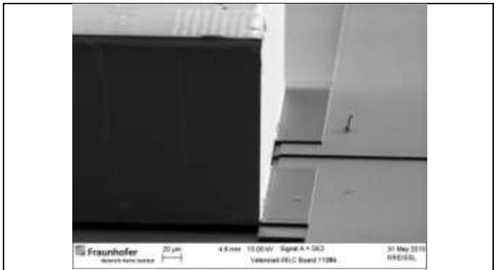
Fig. 13 Placement in direction of optical axis, misalignment ~1 micron
