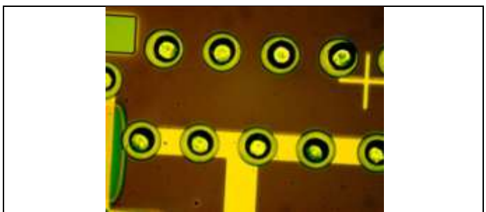
Fig. 14 Microscope image of solder bumps deposited by ejection bumping on SOI motherboards. The bumps are about 40 \mu m in diameter, the pads have a diameter of 60 \mu m.
