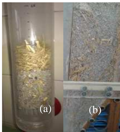
Figure 2.7. Segregation in a standard fluidisation reactor (a) and in a spouting bed reactor (b)
