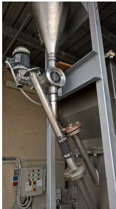
Figure 5.5. Feeding system after the modification on the initial design
