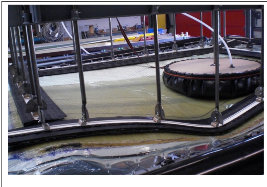
Figure 9: The mould during an injection
