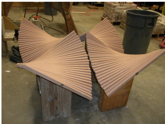
Figure 9. Four hypars making up roof
