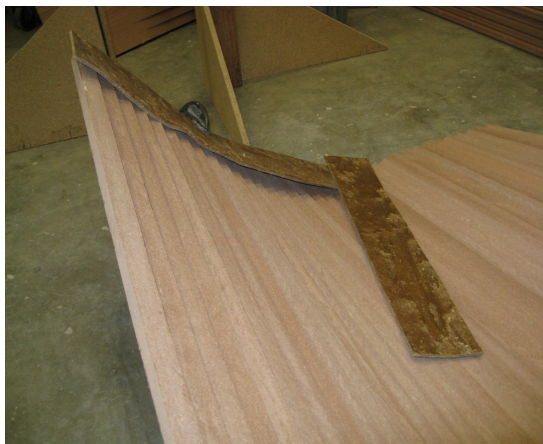
Figure 15. Thin strip following hypar
