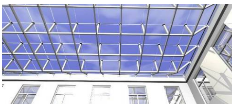
Figures 8a and 8b: Pictures of the film sequence with structure half-Vierendeel
