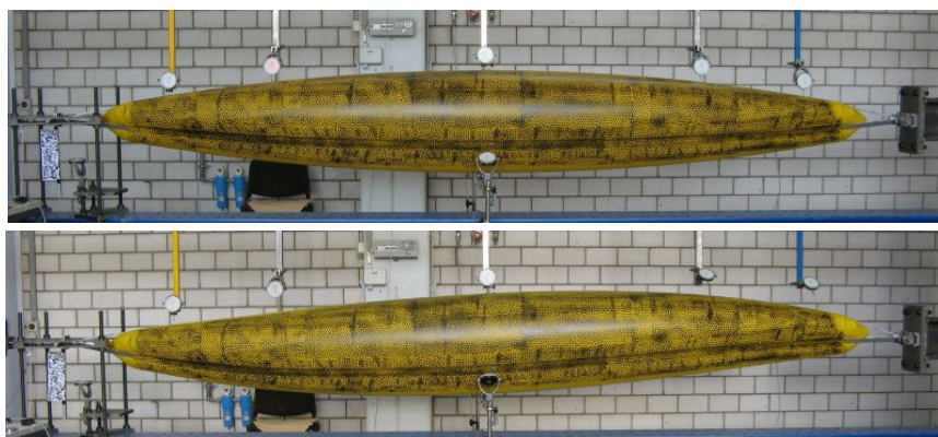
Figure 8: Web-spindle before loading (top) and after buckling in a global 2 nd order mode (bottom)
