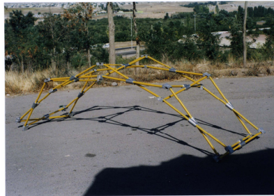
Figure 16: Barrel vault foldable structure
