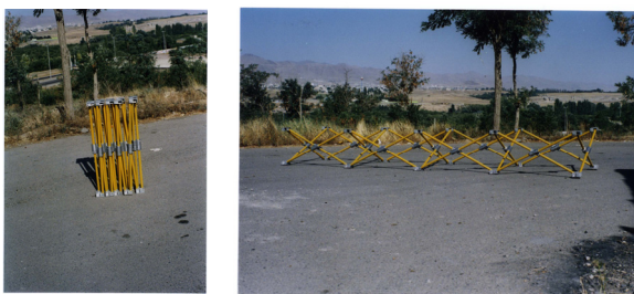
Figure 15: Flat foldable structure in the folded and fully deployed configurations
