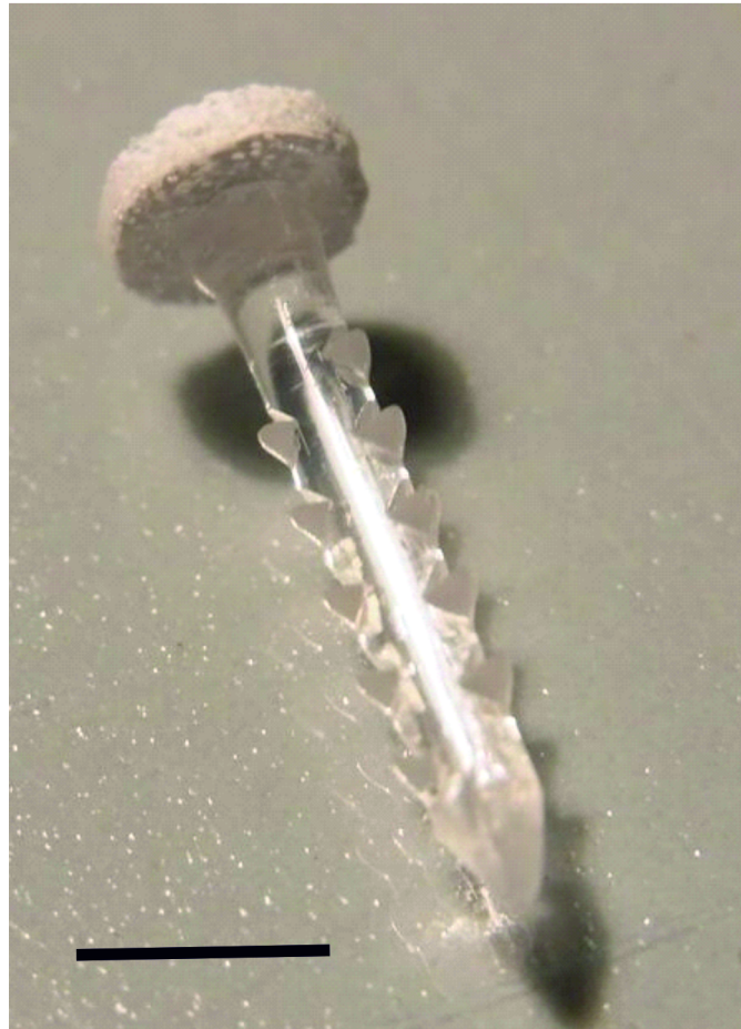
Figure 1. The implant device employed in the second trial group, consisting of a porous PCL scaffold attached to a PLLA pin. Scale bar 4 mm.
