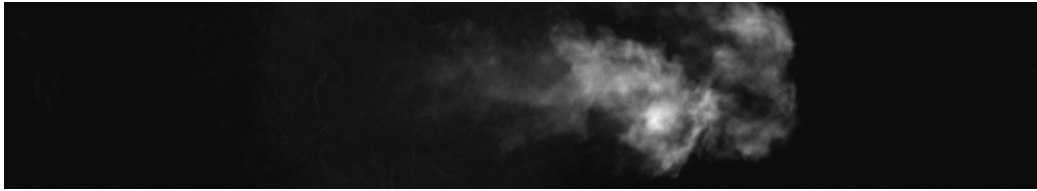
Figure 3: Sample of the broadband radiation imaging at 3000\mu s after SoI
