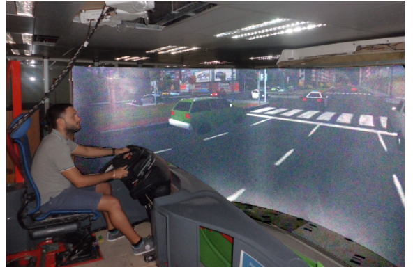
Figure 11. Driving simulation cabin with projection system composed by 3 projectors and a semicircular screen.
