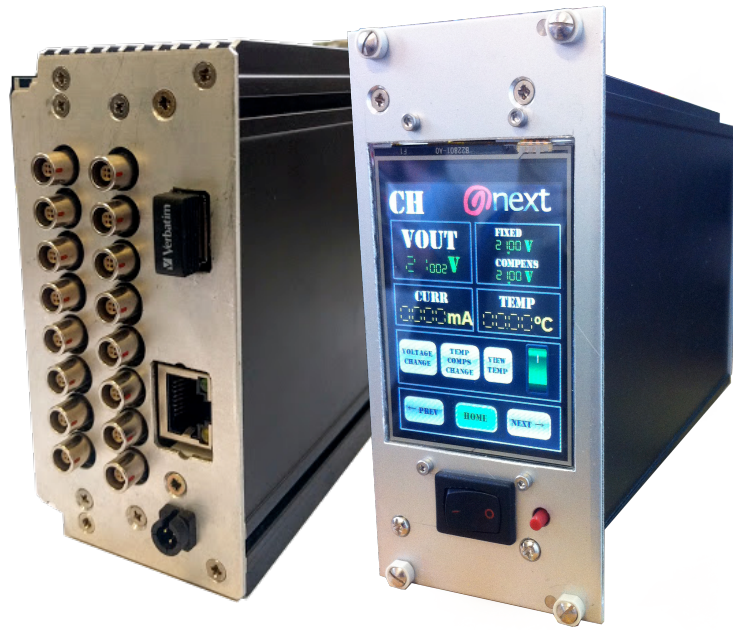
Figure 3. The SiPM power supply for the NEXT experiment, front and rear views. It is a 3U rackable unit with (front) touch screen, on/off switch, reset button and (rear) 16 4-pin LEMO connectors, \pm 12\text{V} power input, Ethernet and USB connectors.
