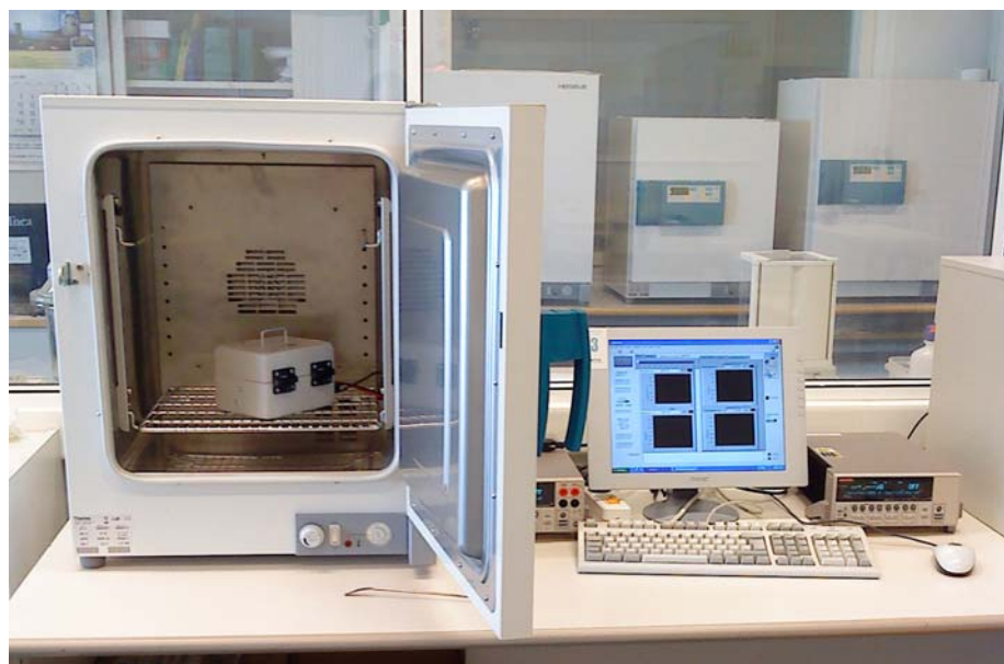
Figure 8.2 Test fixture to test polarisation and depolarisation curves
