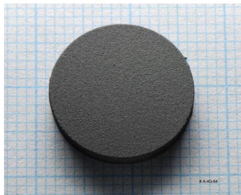
c) Coating on 'as-annealed' support. After annealing in Air at 900°C .
