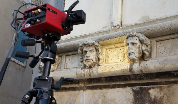
Figure 1: The scanning process of two heads from the Cathedral of St. James in Sibenik, Croatia.
