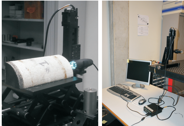
Figure 5.9: Pictures of the PCE-MM200 digital microscope mounted on the guide system.
