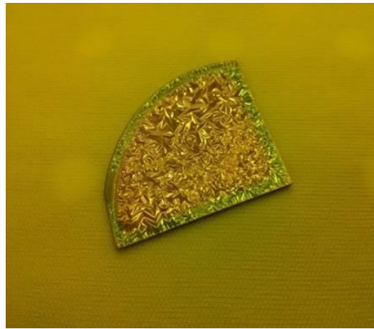
Figure 3.8: Stress problem in sample processed with recipe 2.
