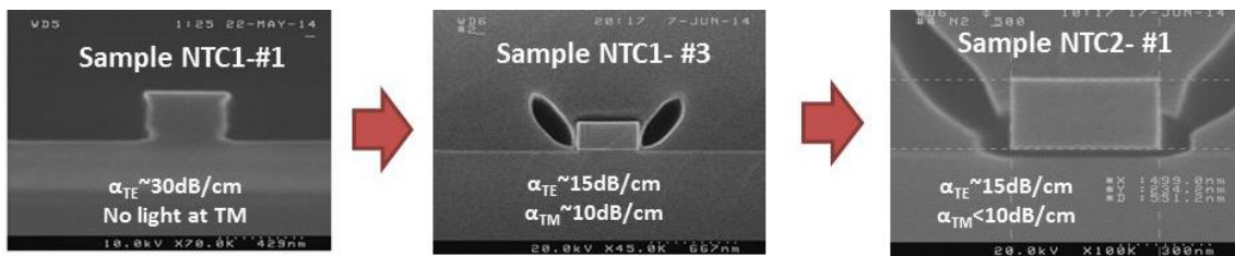
Figure 3.6: SEM images of fabricated a-Si:H waveguides. The waveguide thickness is ~220nm. The waveguide width is 450nm in sample NTC1-#1 and was changed to 500nm in NTC1-#4.
