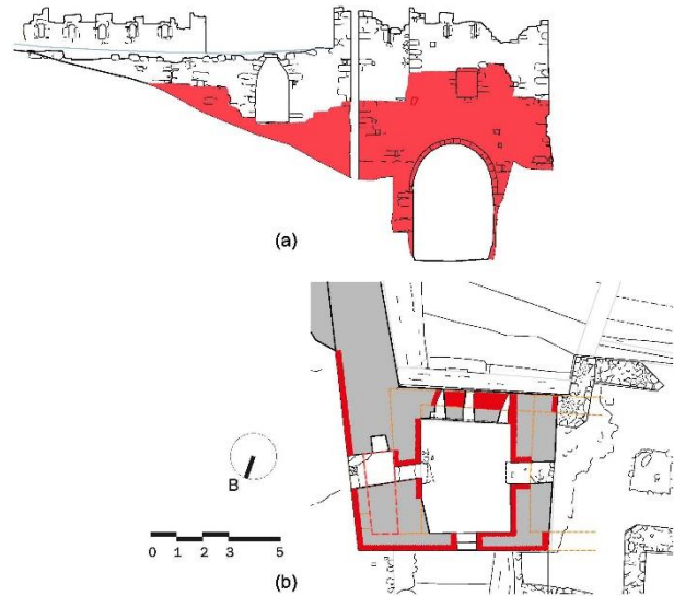
Figure 11: 1 st Byzantine Gate 2D survey: a) Byzantine parts in elevations, internal view; b) ground plan with indications of fragmented Byzantine surface.
