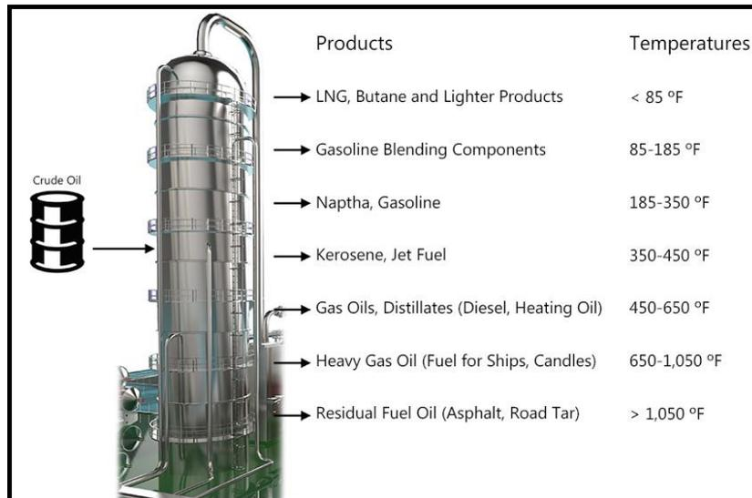
Figure 2-1: Distillation column showing the separation of crude oil into distillates [2.3].
