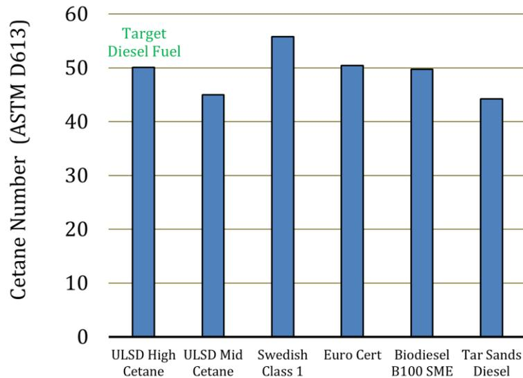
*Figure 5-2: Cetane number measurements of full-range petroleum and biodiesel fuels.*
