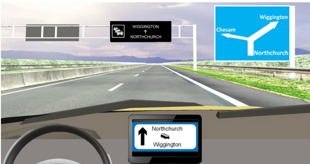
Fig. 3 – Simultaneous display of possible posted, in-car and hybrid VMS signs (II)
