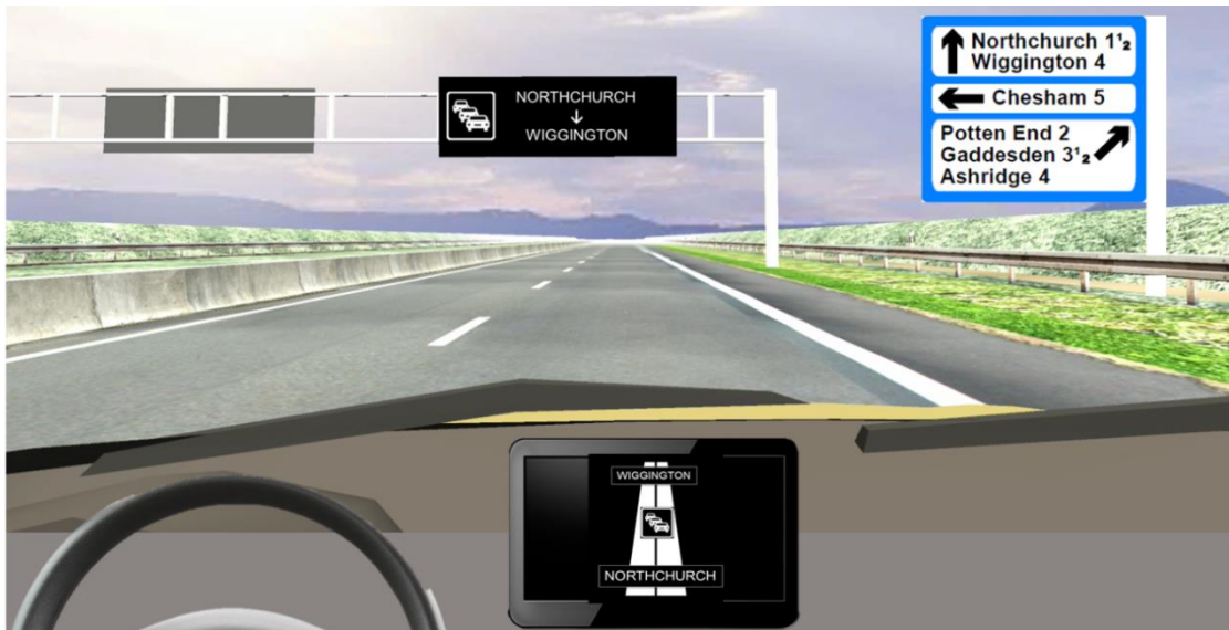
Fig. 2 – Simultaneous display of possible posted, in-car and hybrid VMS signs (I)
