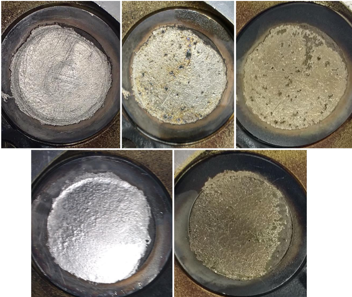
Figure 7-5: Coated Intake Valves, Before and After In-Cylinder Firing Conditions
