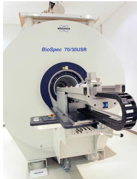
Figure 2.3 Magnetic Resonance scanner at Instituto de Neurociencias in Alicante in San Juan de Alicante (Spain). 7 T MRI scanner (Bruker, BioSpect 70/30, Ettlingen, Germany) used for the acquisition of the data presented in this Doctoral Thesis.
