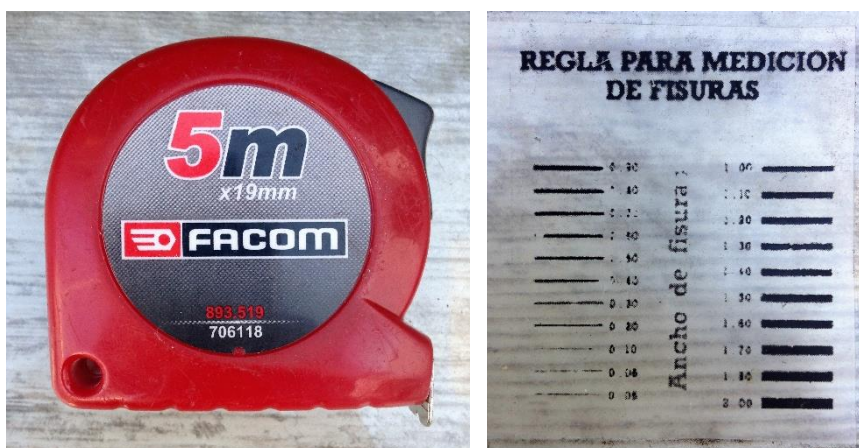
Figure 7.14: Equipment for the measurements of concrete cracks
