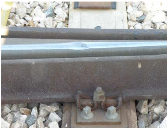
Fig. 7. Squat at the nose of a turnout frog
