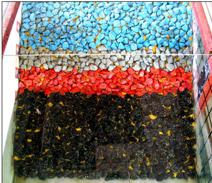
Fig. 3. Frontal view of the breakwater model.
