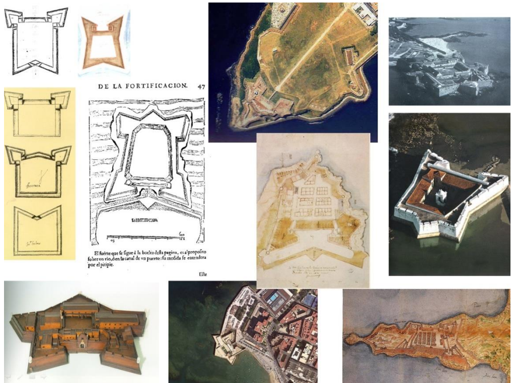
Fig. 5- Comparatives between plain curtains and perced-shaped designs in Escrivá's treatise and "morros" design in Spanish fortification. From left to right, in columns: Design of San Telmo at Malta; proposal of Rojas' treatise (1598); model and aerial view of the fort of Santa Catalina at Cádiz, designed by Rojas too. aerial view of the "Morro de San Juan" at Puerto Rico and plan of La Habana "Morro"; Nowadays views of Blavet castle at Port Louis, France and Natal in Brazil, both from the end of 16th Century. Drawing of 1575 of Mars-El-Kébir fort in Oran.
