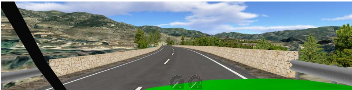
d) Driver's view of a high safety section with walls alienated to the axis of the road.
