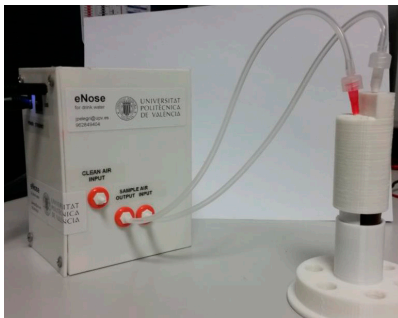
Figure 6. Picture of the low power and low cost MOOSY4 eNose for IoT designed.
