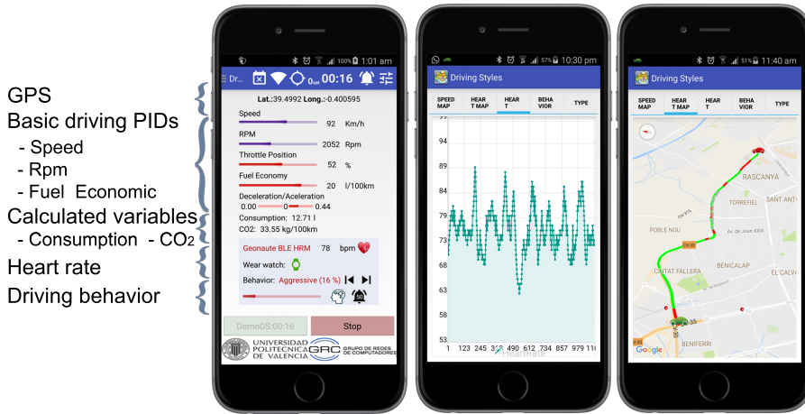
Fig. 3 Snapshots of the main screen and the heart rate module for the Android application.
