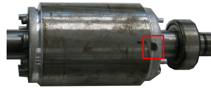
Fig. 13. Rotor with a forced broken bar.
