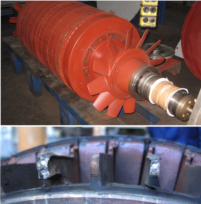
Fig. 1. Top:rotor of the motor of 3.15MW. Bottom: detail of the broken bar.
