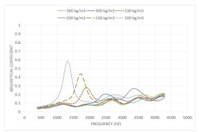
Fig.3. Shows the influence of the density in the sound absorption coeficient in EVA samples of thickness 10 mm.
