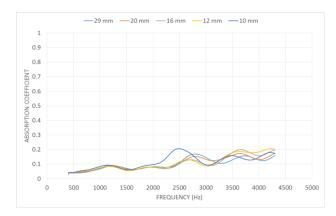
Fig.4. Shows the influence of the thickness in the the sound absorption coeficient in EVA samples of density of 300 kg/m3.
