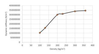
Fig.5. Influence of the density in the dynamic stiffness in EVA samples of thickness 10 mm.
