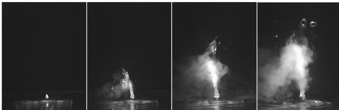
Figure 3. Evolution of the ultrasonic atomization process for increasing voltages. From left to right: 20 V, 30 V, 45 V and 55 V. Atomized liquid is water.
