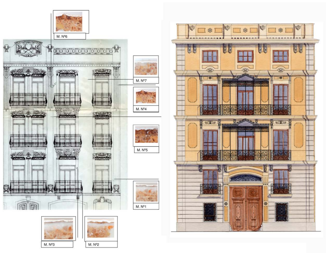
Fig. 4. Chromatic and material study of a facade of the historical center through stratigraphic analysis of plaster samples.
