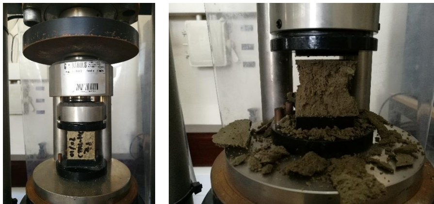
Fig. 3-31. Compressive strength of mortar cubes (left) and CA mortar cube broken at 2 days (right).
