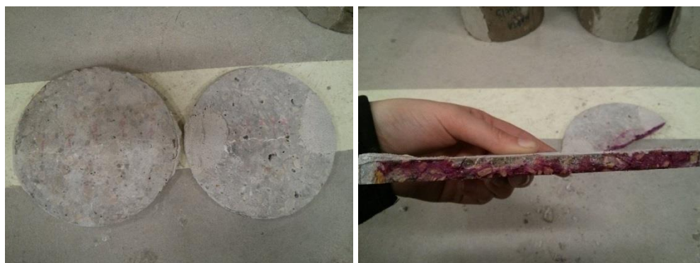
Fig. 5-30. Sealed disks (left) and broken half of a disk after the phenolphthalein test (right).
