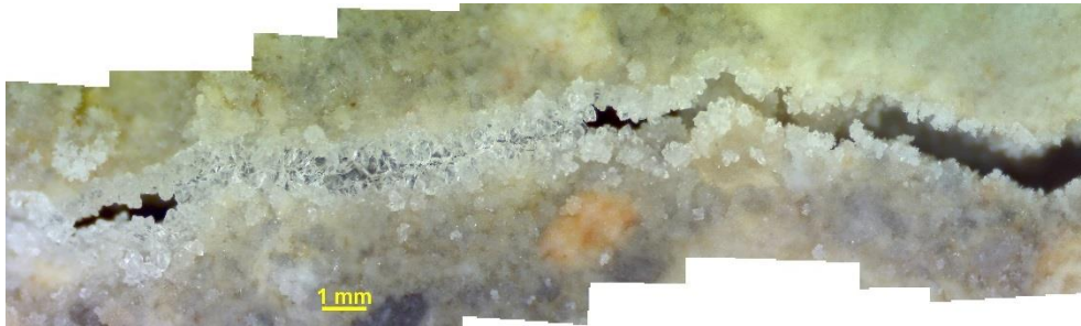
Fig. 4-11. Presence of tooth-like precipitates in specimens healed under water immersion.
