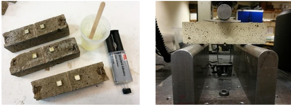
Fig. 3-21. Cleaning steel plates (left) and attachment in the specimens (right).
