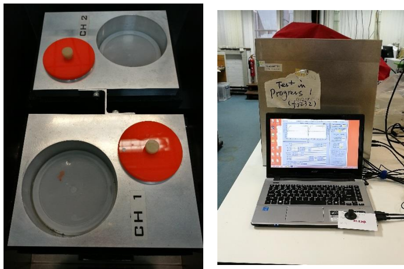
Fig. 3-36. Recipients inside the calorimeter (left) and computer and calorimeter set up (right).
