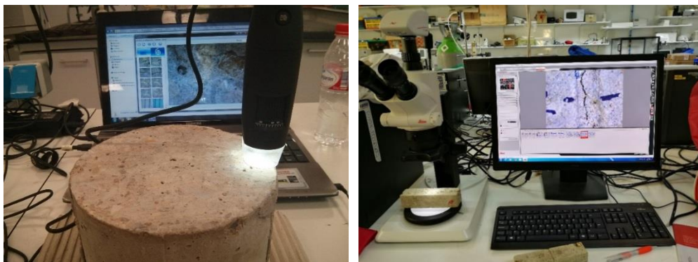
Fig. 3-4. Concrete specimen and optical USB microscope (left) and mortar specimen in the Leica stereomicroscope (right).
