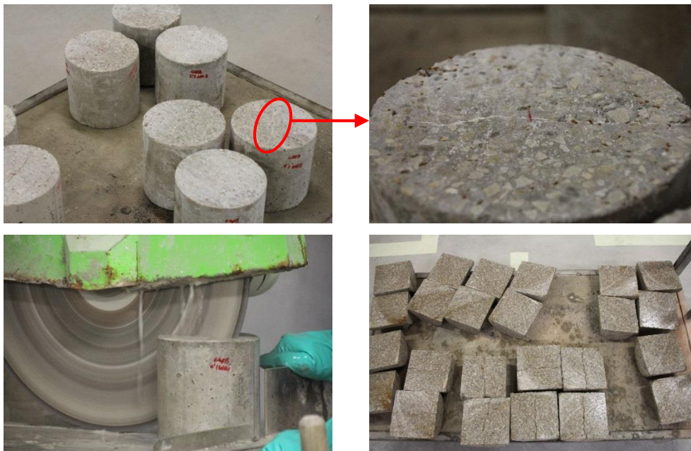
Fig. 5-28. Cutting procedure for concrete specimens
