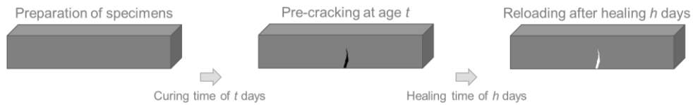
Fig. 3-15. Testing procedure for concrete specimens.
