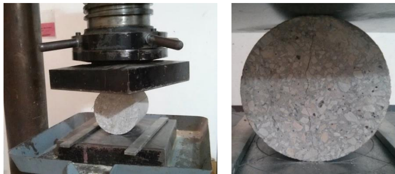
Fig. 3-7. Precracking process and precracked specimen by splitting test.
