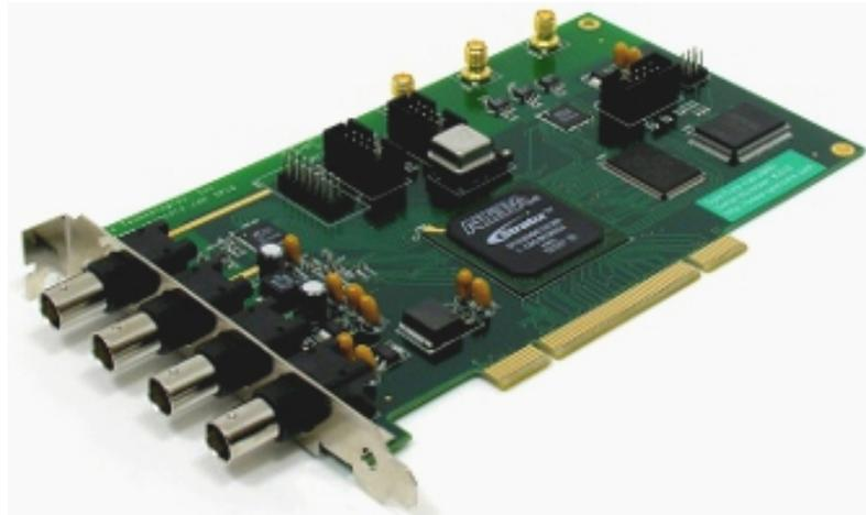
**Figura 4.3:** Tarjeta RadioProcessor-G de SpinCore Technologies Inc. [Spi].
