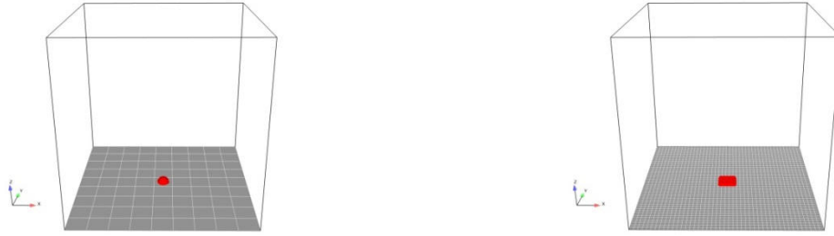
Case (a): Un-resolved liquid film SGS case defined using a single droplet with r_0=1.061\text{ mm} , on one wall-cell face.
