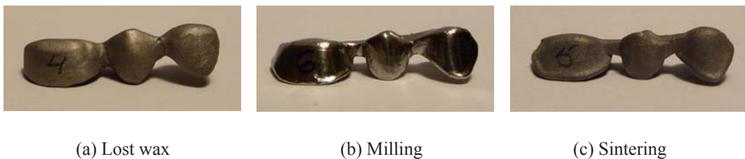
Fig.2. (a) Cr-Co fixed partial denture made using the lost wax technique; (b) milling; (c) selective laser sintering.
