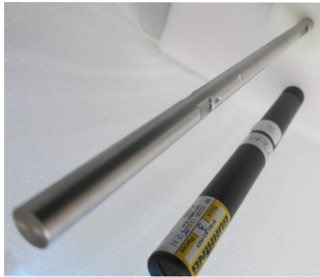
Figure 4.33: Picture of a TZM target prior to irradiation in the HRMT27 experiment. Note that these targets (#1Mo, #2TZM1 and #3TZM2) had a length of 240 mm instead of 140 mm to compensate its longer interaction length due to its lower density
