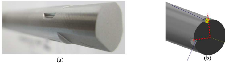
Figure 4.10: (a) Upstream end of an iridium target, including the small slot for the interferometer measurements. (b) Cross-sectioned view of the target in the section where the inclined surface for interferometer measurement were machined.
