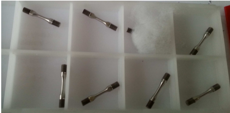
Figure 2.13: Picture of a set of 8 miniaturized specimens -19.5 mm length- of pure iridium as received from manufacturing, before dynamic testing.
