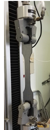
Figure 7.2: Tensile true strain-stress curve of a single sheet of EG of -2.5 mm thickness-tested on its plane direction (see picture in the right).
