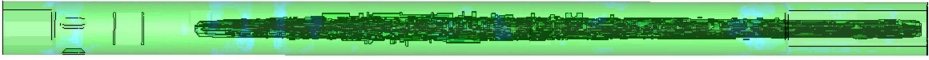
Figure 4.8: Estimation of failure of a tungsten HRMT27 target at conditions reached in the AD-Target core assuming W and a Minimum Hydrostatic Pressure failure model with a failure threshold of 2.6 GPa.
