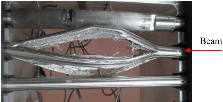
Figure 5.20: Picture of the state of the #12Ir3 target after a single beam impact of 1.71 \cdot 10^{12} ppp.
