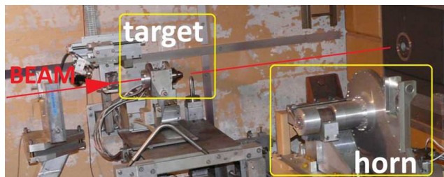
Figure 1.9: Picture showing the current AD-Target and magnetic horn. The proton beam comes from the left of the image and collides with the target. It must be mentioned that in the picture the horn is transversely displaced compared to the operation position, in which the horn and target are in line with the proton beam, as shown in Figure 1.8 [32].
