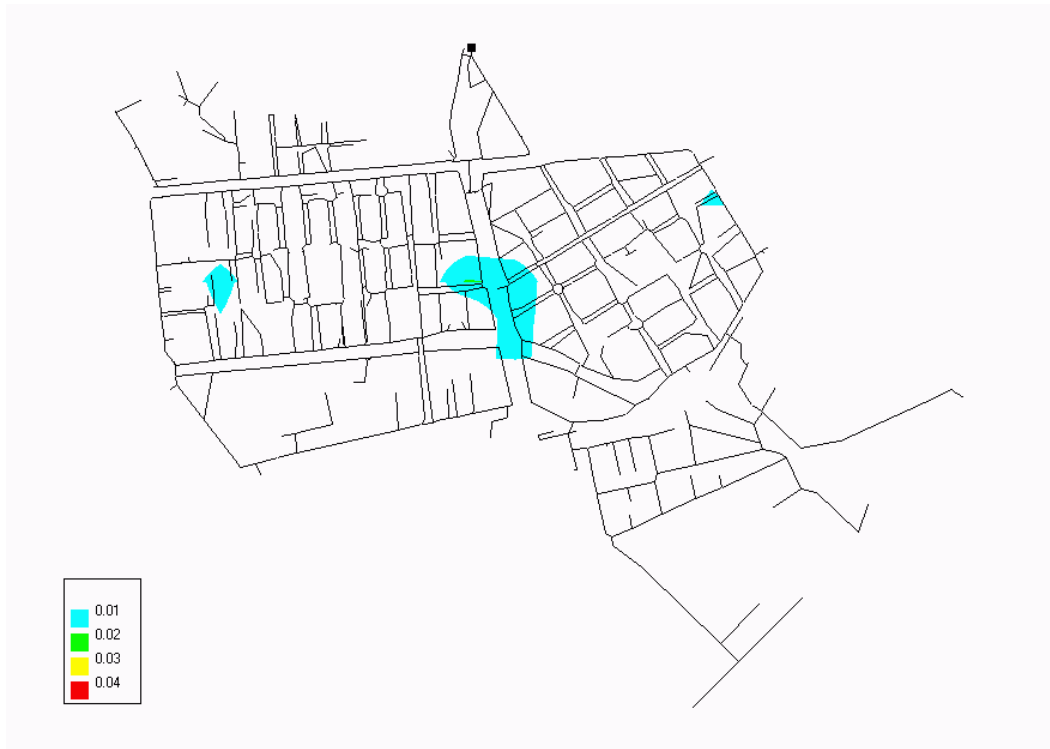
Figure 12: Final leakage distribution (liters/sec) in test 4 (at 0:00 hours).
