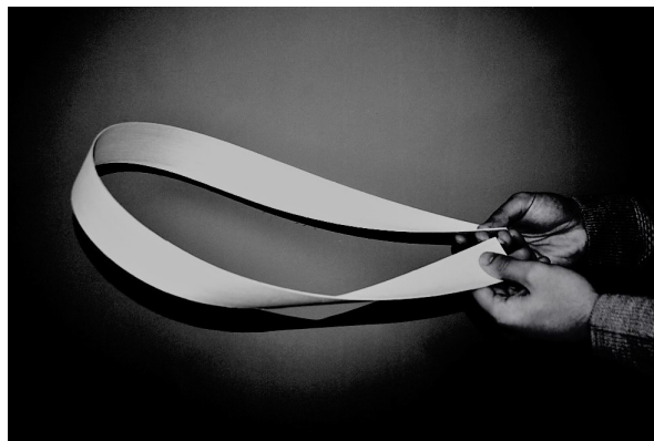
Figure 1: A physical model subject to bending and torsion effects. (Bending of developable surfaces has been studied in [20].)
