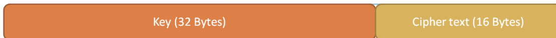
Structure of the command APDU sent to the smart card (Decrypt class)
