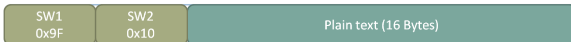
Structure of the response APDU received from the smart card (Decrypt class)
