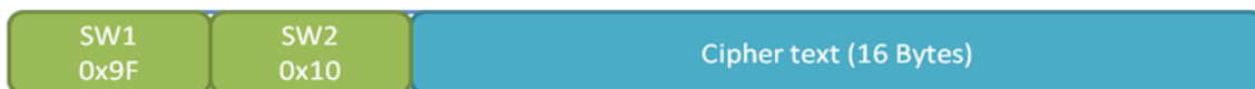
Structure of the response APDU received from the smart card (Encrypt class)
