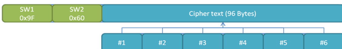
Structure of the response APDU received from the smart card (Encrypt2 class)
