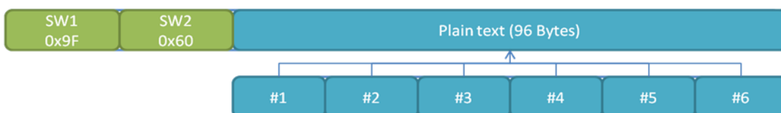
Structure of the response APDU sent from the smart card (NoEncrypt class)
