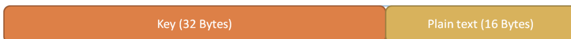
Structure of the command APDU sent to the smart card (NoEncrypt class)
