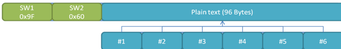
Structure of the response APDU sent from the smart card (NotEncrypt2 class)
