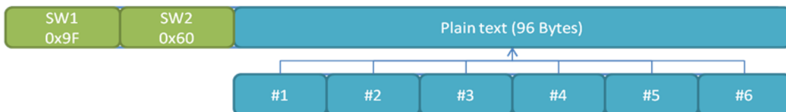
Structure of the response APDU received from the smart card (Decrypt2 class)
