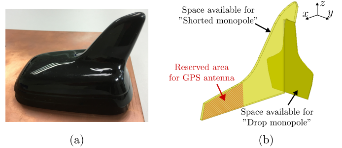
Fig. 1: Configuration of the proposed antenna: (a) Plastic cover (shark-fin), and (b) Parts of the structure.
