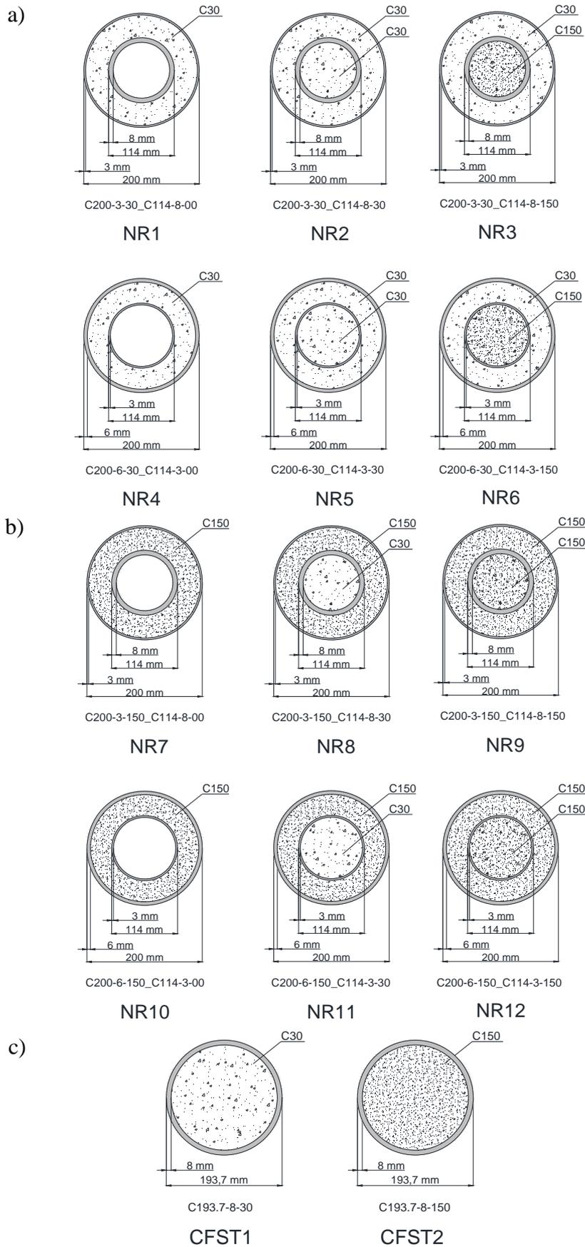
Fig. 2. Room temperature tests: a) Series 1. Outer ring C30 b) Series 2. Outer ring C150 c) CFST specimens
