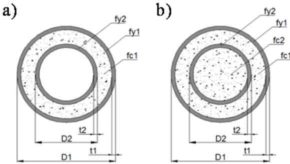
Fig. 1. CFDST sections: a) Double-skin b) Double-tube
