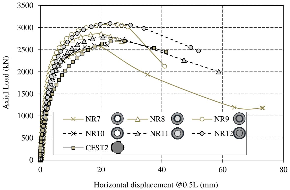
Fig. 6. Axial load versus mid-span displacement in Series 2 (UHSC outer ring).
