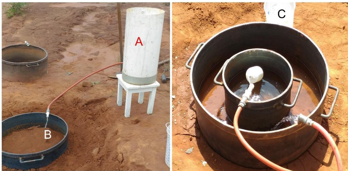
Fig. 3.3 A) Mariotte tube; B) outer ring infiltrometer during installation; C) double-ring infiltrometer test in progress
