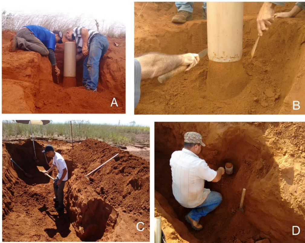
Fig. 3.1 A) Extraction of a large-scale undisturbed soil sample (0.45 m height and 0.20 m inner diameter) from a slope. B) Extraction of a large-scale undisturbed soil sample (0.60 m height and 0.15 m inner diameter). C) Ditch opened to take small-scale samples. D) Extraction of a small-scale undisturbed soil sample (0.15 m height and 0.10 m inner diameter) from the ditch
