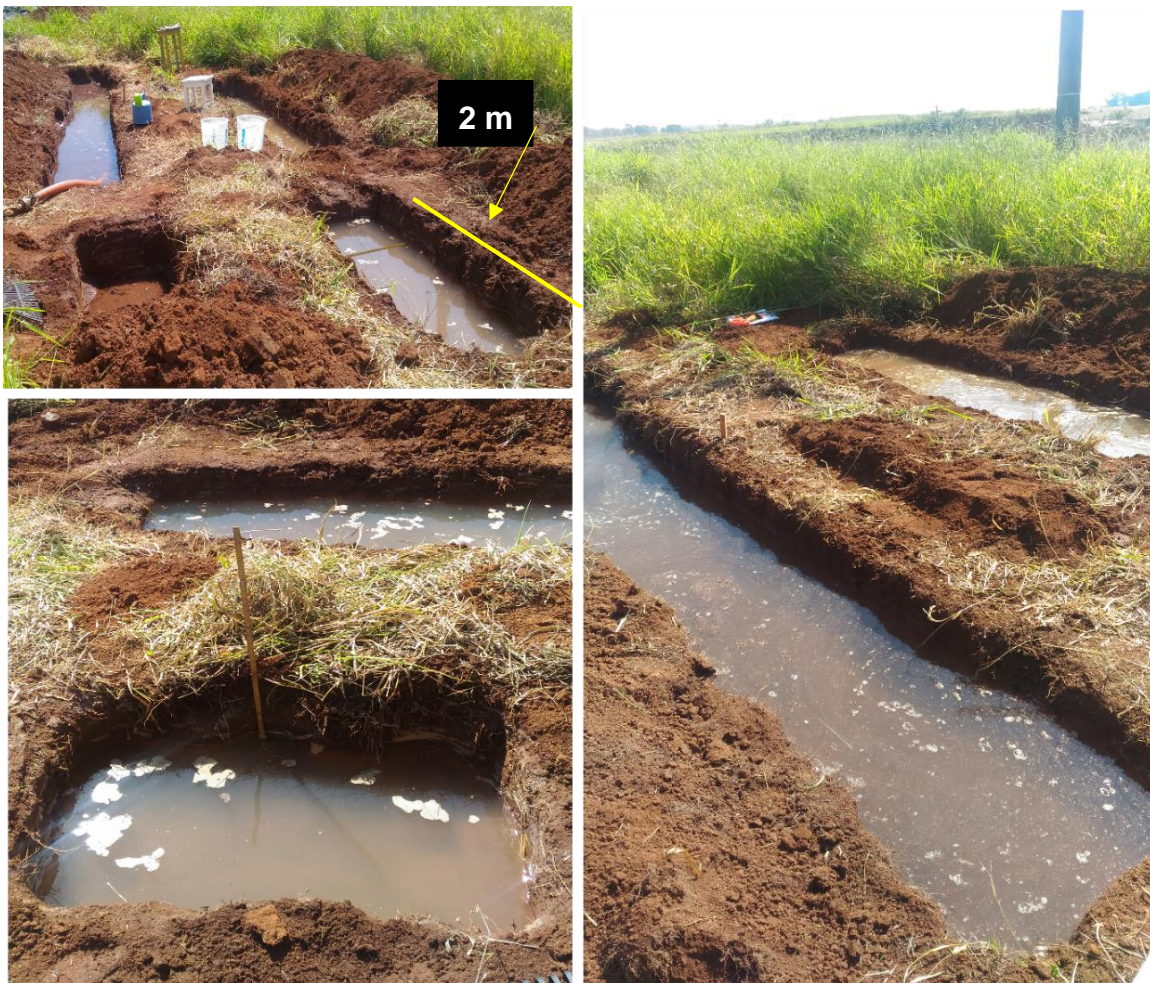
Fig. 3.5 Infiltration in rectangular ditches in progress
