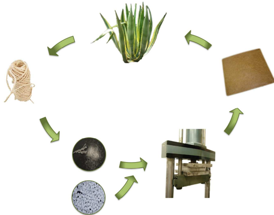
Figure 1. Schematic illustration of the sustainable closed-loop model for the green composites described in this research work: Compression-molded sheets are fully obtained from natural resources and finally converted to compost for the new plant to start the cycle again.
