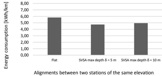
Figure 7. Total energy consumption in the hypothetical vertical alignments
