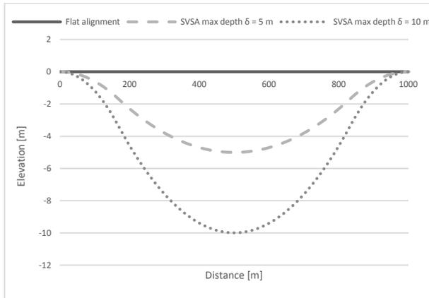
Figure 6. Hypothetical scenarios of vertical alignments between two stations of the same elevation
