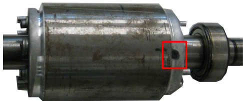
Fig. 6. Rotor with an artificially broken bar used in the experimental tests.
