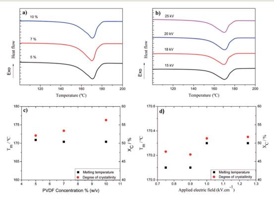
Fig. 7 DSC thermographs of the PVDF microparticles obtained from (a) 5, 7 and 10 (% w/v) polymer solutions and (b) at different applied electric fields. Variation of the sample melting temperature and degree of crystallinity with (c) the solution concentration and (d) applied electric field, respectively.
