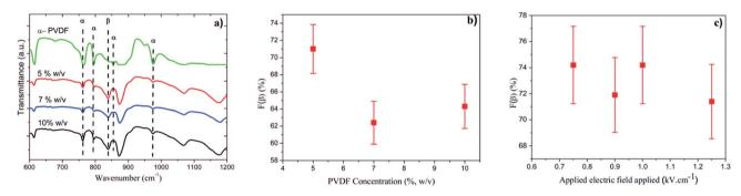
Fig. 6 (a) FTIR spectrums of 5, 7 and 10 (% w/v) PVDF microparticles and  $\alpha$ -PVDF film; (b) the variation of  $\beta$  phase content with the concentration and (c) with the applied electric field for 5 (% w/v) samples.
