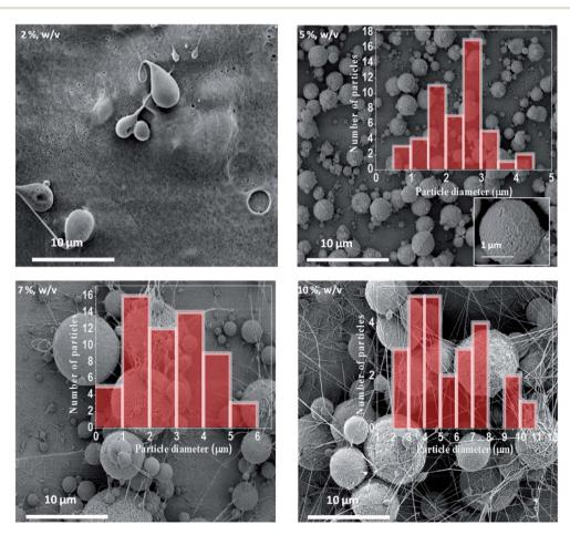
Fig. 1 Morphology of the PVDF microparticles for the samples obtained with 2 (a), 5 (b), 7 (c) and 10 (% w/v) (d) polymer solution obtained at an applied electric field of 1 kV cm $^{-1}$  with a needle diameter of 0.2 mm, flow rate of 2 mL h $^{-1}$ . The microparticle distribution obtained from each processing condition is presented as an inset.
