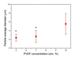
Fig. 2 Influence of the PVDF solution concentration (% w/v) on microparticle average diameter. The bars in the graph are the standard deviation of the fiber diameter distribution. \* $P \le 0.05$  vs. PVDF concentration of 10 (% w/v).
