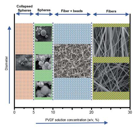
Fig. 5 Schematic diagram of the influence of PVDF solution concentration in the production of microparticles and fibers by electrospray.
