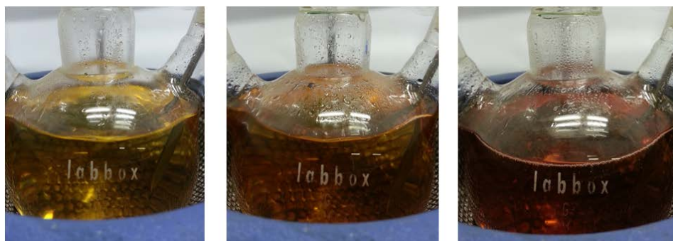
Figure 3.- Influence of the reaction temperature and time on the colour during maleinization process of cottonseed oil, a) 180 °C – 60 min, b) 200 °C – 60 min, c) 220 °C – 60 min.
